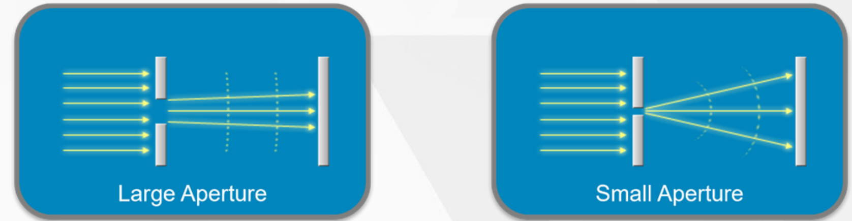
Diffraction depending on lens aperture
