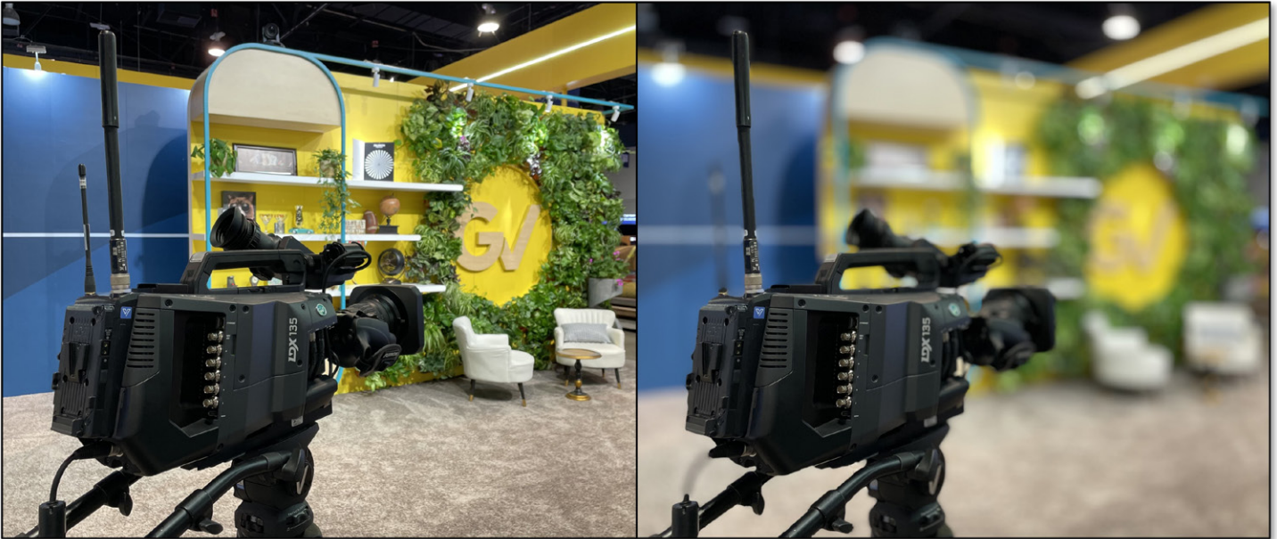
Figure 1 – Comparing large depth of field and shallow depth of field (simulated image)
