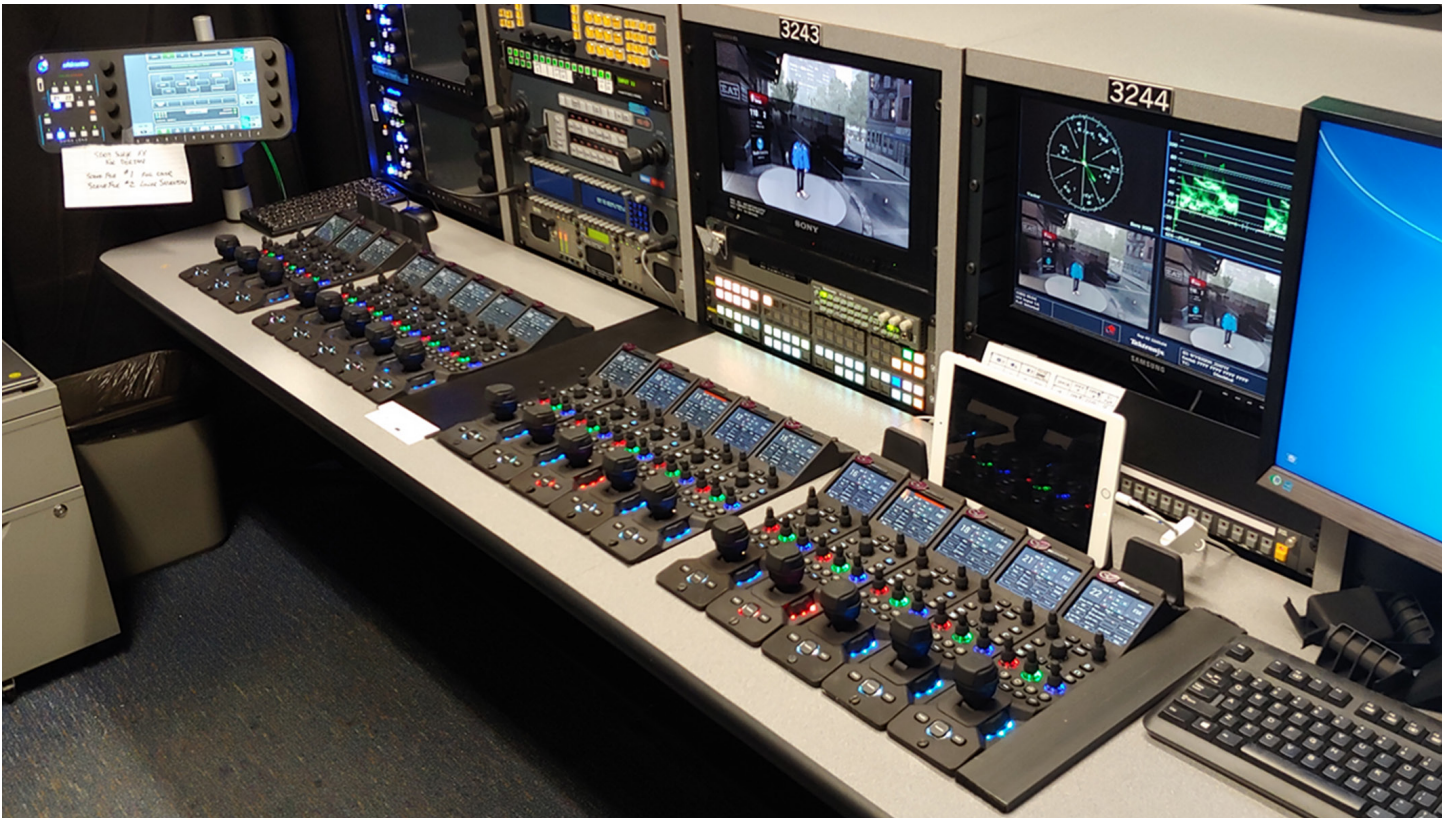
Figure 7 – Camera shading solution with advance features for live applications
